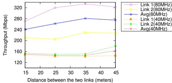
Fig. 9: Two 802.11ac links - comparison of interference pattern between two cases, case 1 when both links operate on 80 MHz and case 2 when both links operate on 40 MHz.
