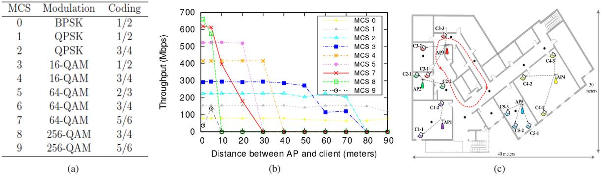
Fig. 1: (a) 802.11ac MCS index table, (b) Throughput with different MCS values when SS = 3, (c) Testbed of 18 802.11ac nodes used for the experiments.
