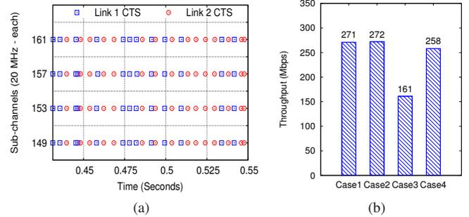
Fig. 8: (a) RTS-CTS packets captured by sniffer (b) Throughput comparison of 4 cases where two links (Case-1): share 80MHz with same primary channel, (Case-2): share 80MHz with different primary channel, (Case-3): divide 80 MHz into adjacent 40MHz channels, (Case-4): divide 80 MHz into non-adjacent 40MHz channels
