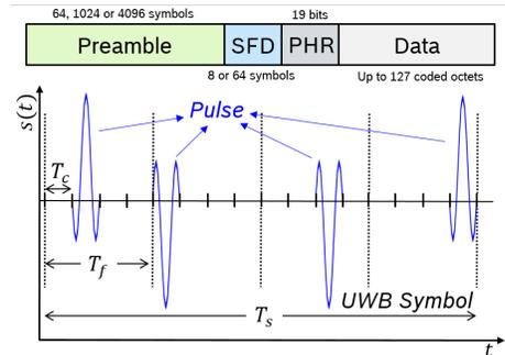
Fig. 3: UWB packet and UWB symbol structures.
