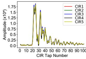
Fig. 9: Each receiver performs CIR alignment by identifying the tap corresponding to the first path, and shifting it to a pivot tap.
