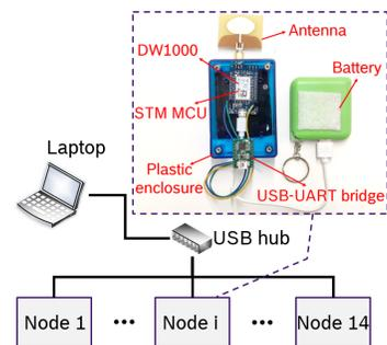
Fig. 17: *CaraoKey* node and data collection system architecture.
